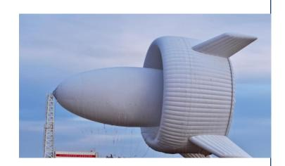
costs by 30% compared with traditional land-based wind turbines. The S1500 is designed for rapid deployment in remote areas or during emergencies. The entire unit can be moved within hours, making it suitable for deserts, islands, and mining sites.
