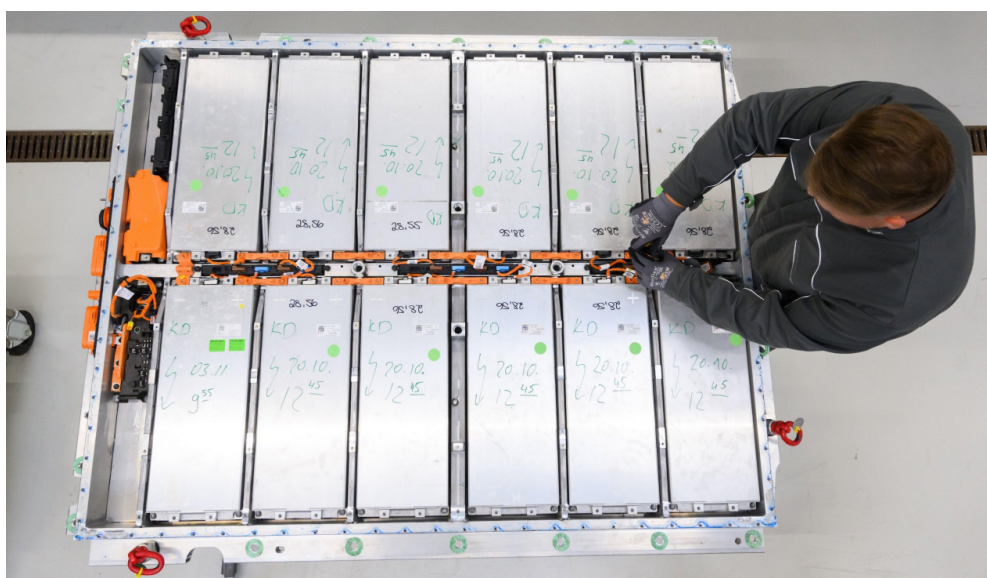
An employee removes modules from a worn-out EV battery at the Volkswagen plant, Salzgitter, Germany
