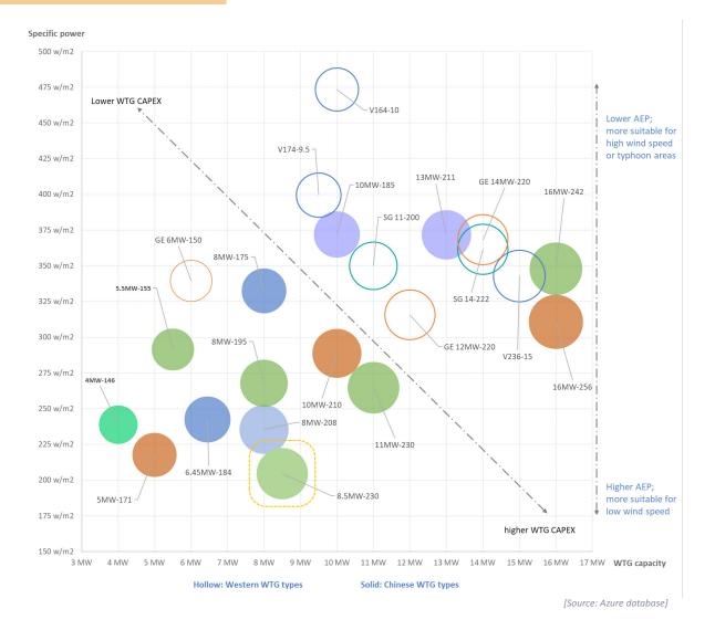
It can be easily imagined that larger rotors produce more power for a given turbine capacity, but they also have drawbacks such as severe loading on both turbine and foundation, as well as logistical and installation challenges. The table below provides a high-level comparison of each type's advantages and drawbacks.
