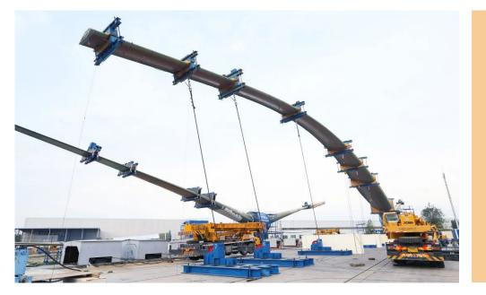
YD110 blade under static loading test per IEC61400-23.
