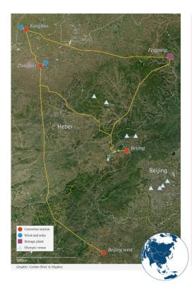
An approximate map of the green electricity grid connecting wind and solar power in the western part of Zhangjiakou to the Fengning pumped storage station and to a converter station near Beijing. There are two converter stations with dedicated wind and solar capacities in Zhangjiakou. The locations of the Olympics venues are shown as well. Source: Project maps for the Zhangjiakou green grid and the Zhangbei-Xiongan UHV line.
